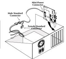
Converter. Attach the male end of the "Y" connector to a standard size power connector in your computer. Replace the cover. Attach the cables between PC Media Converter and the devices that will be interconnected.
