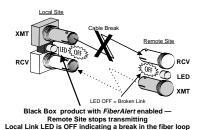
status of the opposite end of the fiber. Both fiber link LEDs on either end of the link should extinguish, alerting you to the fault.
