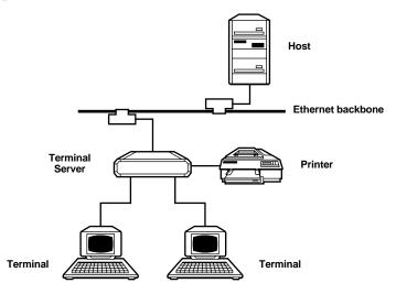
Figure 3-1. A Typical Terminal Server Layout.
