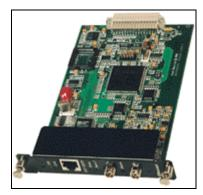
Figure 1 - CityLIGHT 10/100 Ethernet Transceiver
