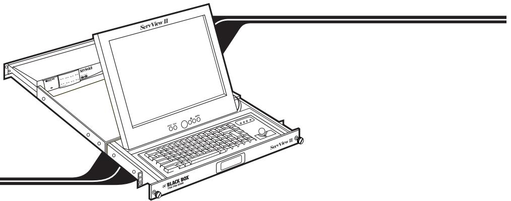
The ServView II is a rackmountable KVM tray that contains a Cherry<sup>®</sup> keyboard and trackball and the thin-film transistor (TFT) display of a Samsung<sup>®</sup> SyncMaster<sup>®</sup> flat-panel monitor. Most models also include an 8-port slimline version of one of our ServSwitch<sup>™</sup> brand KVM switches. There are five models of the ServView II:
