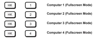
Press hotkey followed by 1, 2, 3 or 4 to switch the corresponding computer to Fullscreen mode and enable its keyboard and mouse.
