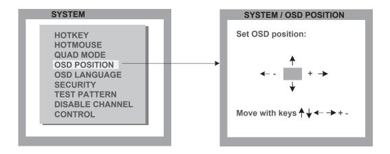
Use this function to move the OSD window to any position on the screen.
