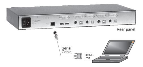
Use the serial cable to connect the COM port of the Windows computer with the serial port of your ServSwitch 4site.
