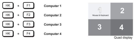
Simultaneously press hotkey and F1, F2, F3 or F4 to switch to Quad mode and enable mouse and keyboard of the computer in the respective quadrant.
