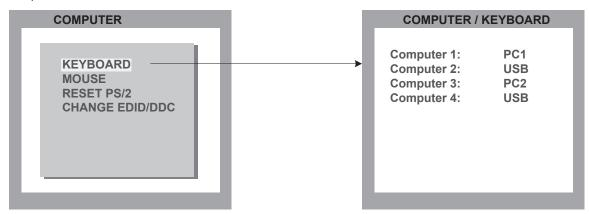
Use this display feature to identify which keyboard type (USB, PC1, PC2 or PC3) has been recognized at which computer port.
