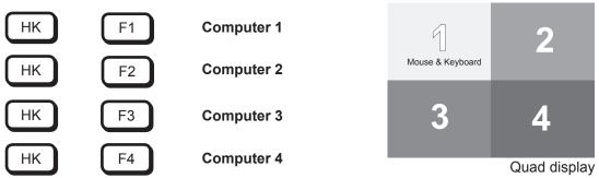
Press hotkey followed by F1, F2, F3 or F4 to switch to Quad mode and activate mouse and keyboard of the computer in the respective quadrant.
