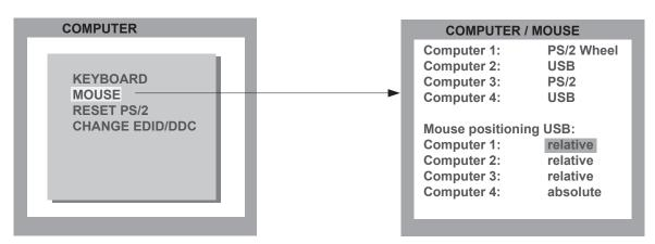
The upper half of the MOUSE window shows which mouse type (USB, PS/2 or PS/2 wheel) has been recognized at which computer port.
