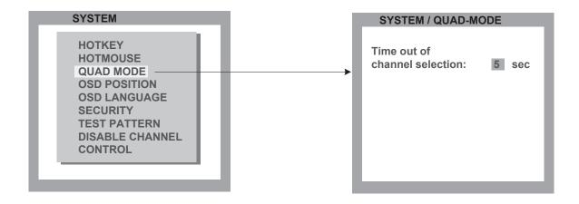
Channel selection timeout defines the period (1 to 30 seconds) after which the selector will close automatically. Default setting is 5 seconds.
