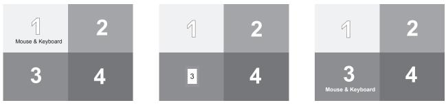
Example: Switch active channel from 1 to 3
