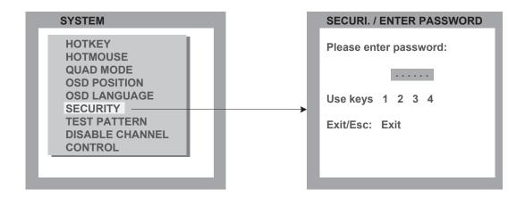
The SECURITY feature allows you to reduce the functional range of the ServSwitch 4site. Eight security levels are available for this purpose.
