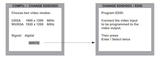
When the window shown on the right opens, connect the video output to the video input to be programmed with a DVI video cable.
