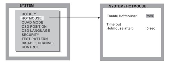
To activate Hotmouse operation, navigate to "Enable Hotmouse" and change the setting to "Yes".
