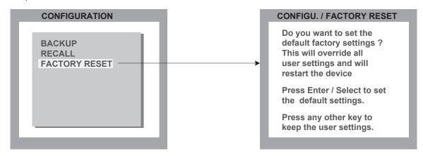
Use this function to reset the ServSwitch 4site to its default settings. If necessary, save your current settings before using the DEFAULTS command. Execution of this command results in a complete reset and reboot of the ServSwitch 4site with factory defaults.
