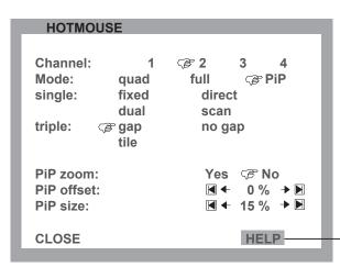
The hand symbol points to the current settings for the active channel, the display mode, and the PiP function.
