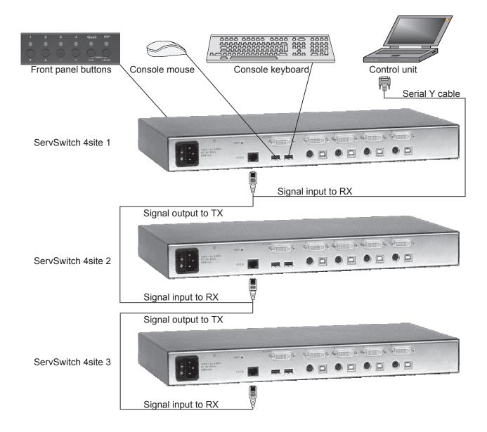
To synchronize, ServSwitch 4site 1 sends every change in settings as a DCP message via the serial Y cable to the RX input of ServSwitch 4site 2.
