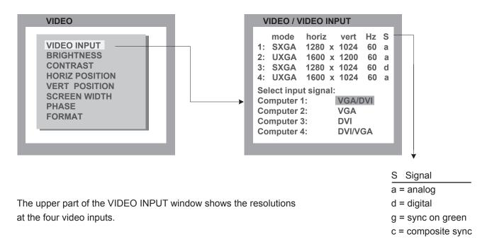
Resolution recognition at the four video inputs is automatic.
