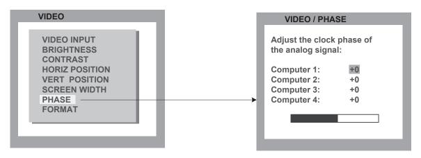
Incorrect phase (sampling time of pixel color value) may result in blurring, bad contrast, or poor legibility. Use this setting to adjust phase.
