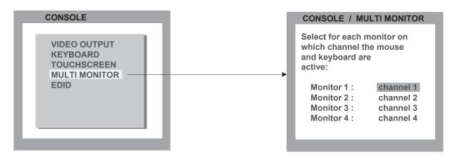
If you use graphics cards with multiple video outputs, you must assign the computer's mouse and keyboard to the corresponding video output (channels 1-4).
