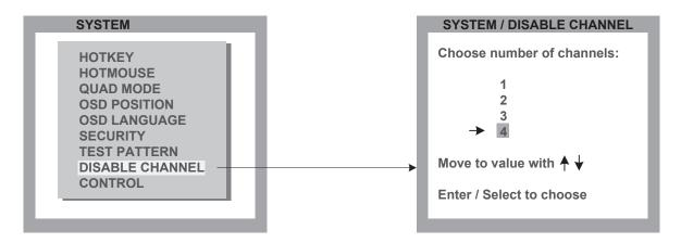
If only two or three computers or video sources are connected to ServSwitch 4site, use the DISABLE CHANNEL feature to ensure that for the unused channels:
