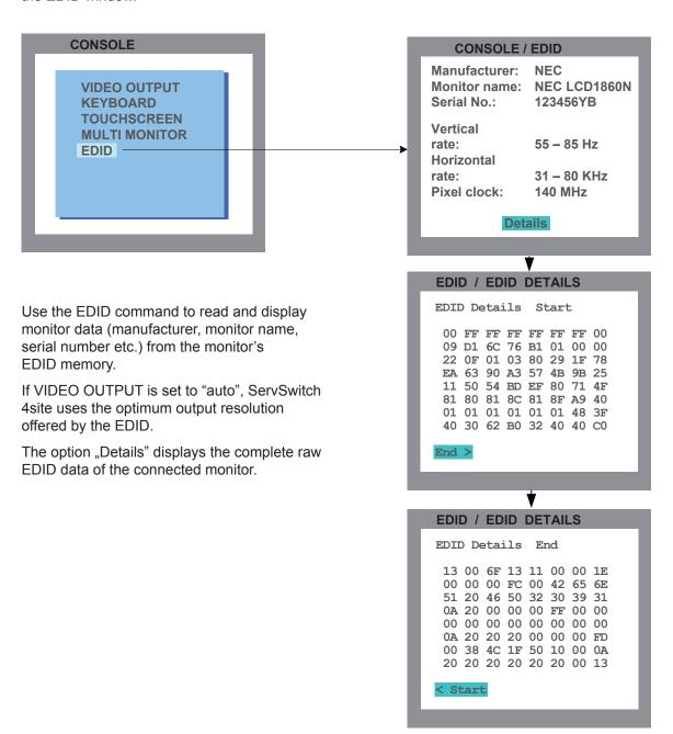
**EDID** (Extended **D**isplay Identification **D**ata) is a VESA standard data format that contains basic information about a monitor and its capabilities. This information is stored in the monitor by the manufacturer and can be read by ServSwitch 4site or graphics card via a monitor cable's Display Data Channel (DCC) interface.
