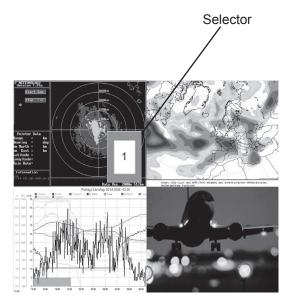
In Quad mode, use **hotkey** 'P' to open the selector. The selector indicates the active channel (mouse and keyboard enabled).
