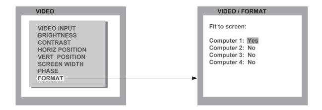
When using a wide-screen monitor (aspect ratio 16:10) in Quad-mode, a video input with a different aspect ratio is normally displayed with black borders to the left and right. If fit to screen is enabled, the image is resized to fill the entire quadrant in Quad mode.
