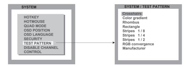
Use the Test Pattern feature to check monitor quality (pixel errors, contrast, etc) or the functionality of the ServSwitch 4site's video output.
