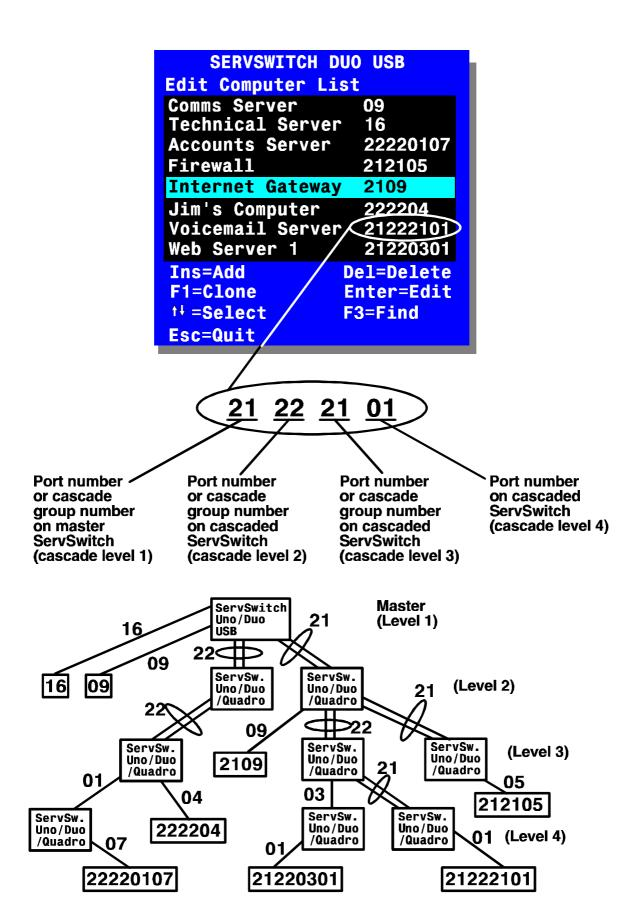
Fig. 6 - Creating menu entries for computers that are connected to cascaded ServSwitches
