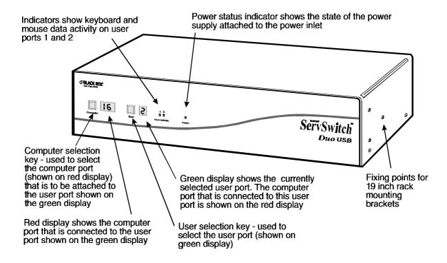
Fig. 1c - KV6616FA ServSwitch Duo USB viewed from the front
