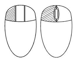
To select a computer in **EXCLUSIVE** mode, use the left hand mouse button together with the SHIFT key on the keyboard. To select a computer in **VIDEO ONLY** mode use the left hand mouse button together with the CTRL key on the keyboard.
