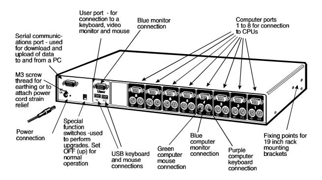
Fig. 2a - KV6508SA ServSwitch Uno USB viewed from the rear
