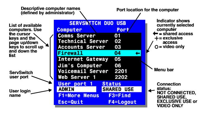
To connect to a computer, place the menu bar over the computer name using a combination of the up and down cursor keys and the page up / page down keys.
