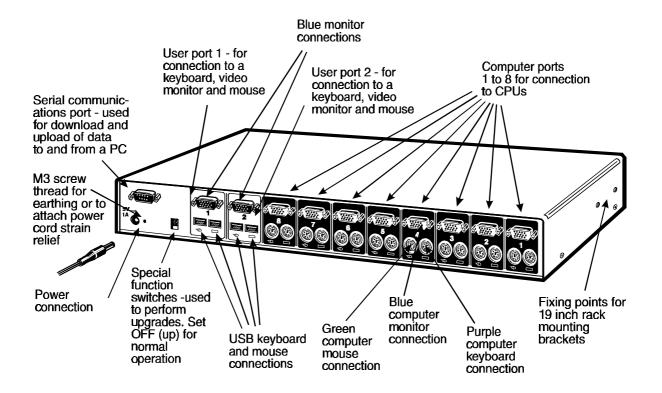
Fig. 2b – KV6608SA ServSwitch Duo USB viewed from the rear
