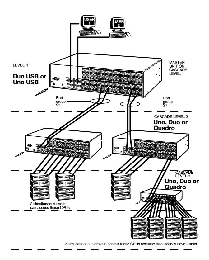
Fig. 5 - A cascaded application using multiple ServSwitch units
