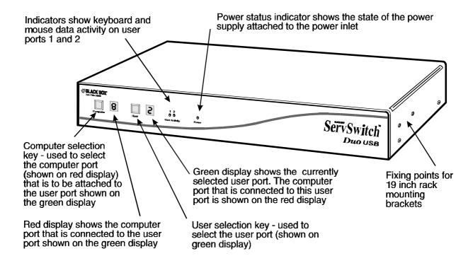
Fig. 1b - KV6608SA ServSwitch Duo USB viewed from the front
