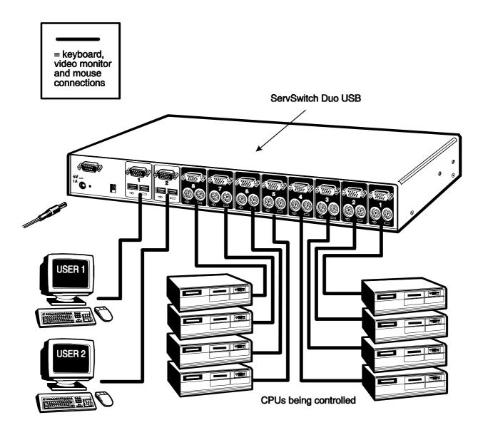
Fig. 4 - A typical installation using a single ServSwitch Duo USB
