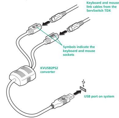
Note: For neatness and accessibility it is advisable to join the keyboard and mouse link cables, that lead to each system, using several cable ties.
