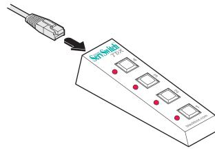
3 At the other end of the cable, attach the larger connector to the socket on the end of the ServSwitch TDX unit.
