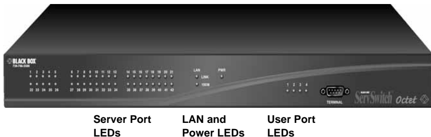
Figure 3-11. Octet Switch LEDs (KV1701A/E Switch Shown)
