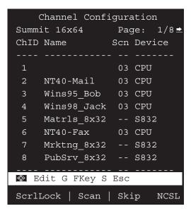
Figure 4-9. The Channel Configuration Menu for a KV1502A (shown after a hypothetical cascaded system configuration is finished).
