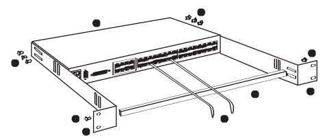
Figure E-3. Rearward rackmounting of the Base Unit (1U model shown).
