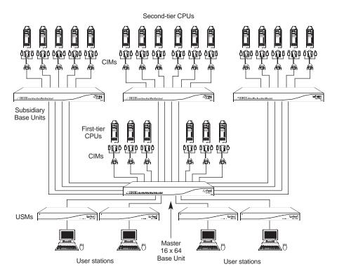
Figure 4-7. A sample cascaded system.
