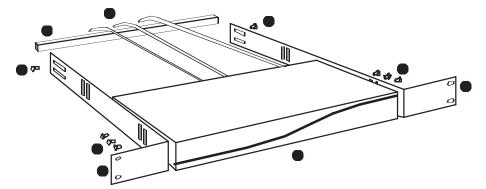
Figure E-2. Frontward rackmounting of the USM.
