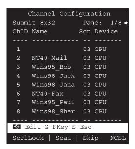
Figure 4-6. The Channel Configuration Menu of a KV1502A (shown after a hypothetical basic system configuration is finished).
