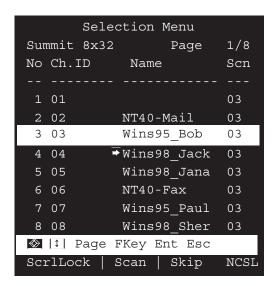
Figure 4-4. The Selection Menu for a KV1502A (shown after a hypothetical basic system configuration is finished).
