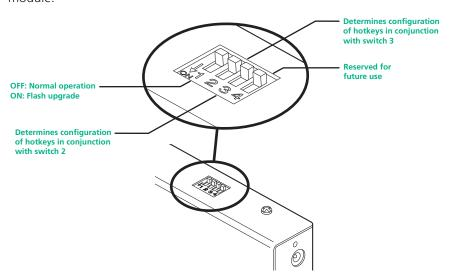
Note: When shipped, all switches are set in the OFF positions and this will produce normal operation.
