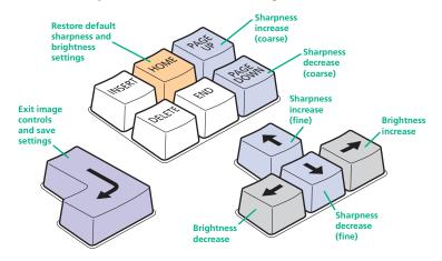
3 When no shadows are visible and the displayed images have crisp edges, press to exit configuration mode and permanently save all settings.
