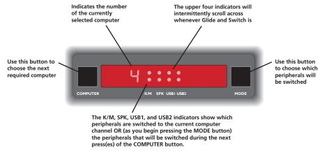
Figure 5-1. Front panel buttons and indicators.
