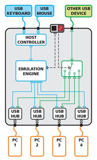
Figure A-1. True Emulation functional block diagram. The emulated section of the switch is shown in blue and handles only the keyboard and mouse. The green enumerated section of the switch handles other USB devices and also uses the USB hubs to link with the computers.
