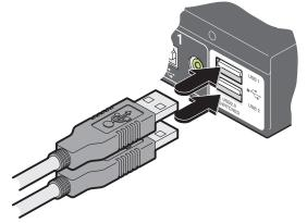
Figure 3-2. Connecting USB peripherals to the user console.
