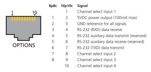
Figure 3-7. Signal and power pin-outs on the OPTIONS port.
