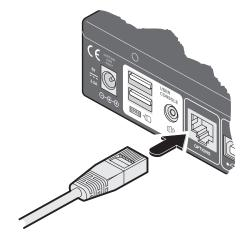
Figure 3-8. Link cable to the OPTIONS port on the rear panel.
