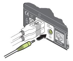
Figure 3-3. Connecting speakers to the user console.
