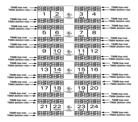
Figure 5. 24-port patch panel's T568B and T568A wiring sticker labels.
