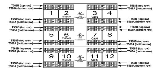
Figure 4. 12-port patch panel's T568B and T568A wiring sticker labels.
