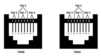
Figure 1. T568B and T568A wiring patterns.
