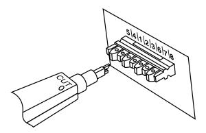
Figure 3-2. Example of module termination.
