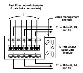
Figure 3-3. Typical setup.
