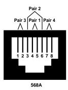
**Wiring** — JPM084A, JPM086A: TS568A (EIA/TIA) wiring pattern; JPM083A, JPM085A: T568B (Bell 258A) wiring pattern
