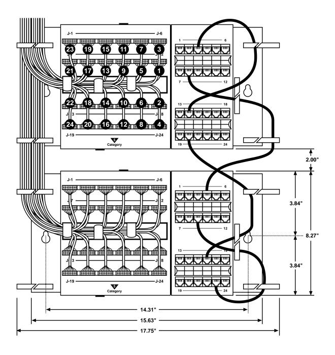
Figure 2. Suggested Cable Installation for the 24-Port Patch Panels.
