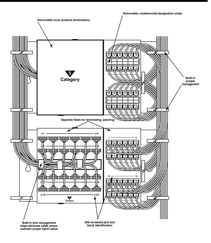
Figure 1. The 24-Port Modular Patch Panel.
