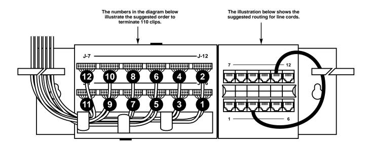
Figure 3. Suggested Cable Installation for the 12-Port Patch Panels.
