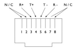
Figure 2a RJ45 Signals (S Interface NT Mode)
