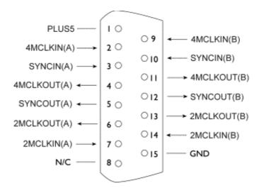
Figure 8 Auxiliary Port Pinout
