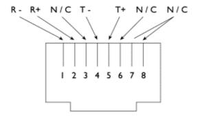
Figure 3b RJ45 Signals (E1/T1 TE Mode)
