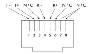
Figure 3a RJ45 Signals (E1/T1 NT Mode)
