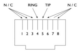
Figure 2b RJ45 Signals (U Interface)
