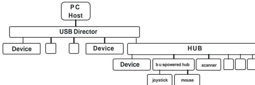
Figure 1: Example of a Typical Hub Configuration
