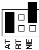
Figure 3-3. Headers J1B – J4B, RS-485 “Auto” Enabled, with “Echo.”
