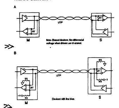
When drivers are tristated, the circuit below is equivalent. Simplification works well for relatively low baud rates.
