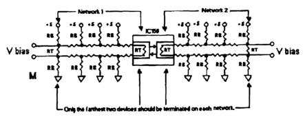
By using the IC158 (Opto-isolated version), total electrical isolation between Network 1 and Network 2 can be established.
