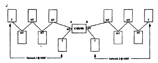
\*\*An important note: Using the IC158 (Opto-isolated version) totally isolates one link from the other (100% electrical isolation).
