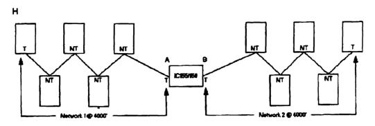
An important note: Using the IC158 (Opto-isolated version) totally isolates one link from the other (100% electrical isolation). Example of extending/bridging a network at the physical end by making the repeater the physical end. (See next diag.)
