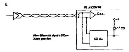
What happens to CD (carrier detect) when Line Bias resistors are added? The answer is CD will always be 'ON'.
