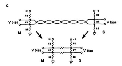
Using devices that have line biasing resistors ensures that a receiver does not see spurious noise on the line as "data" and can make up for a poor cable. But, it also limits the maximum distance and/or the maximum number of "drops" on the network, thus, the need for a repeater function.
