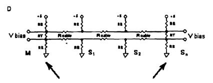
\*ONLY the two furthest devices should be terminated. None in between.\*
