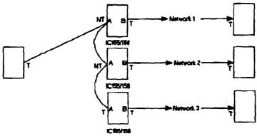
\*\* An important note: Using the IC158 (Opto-isolated version) totally isolates one link from the other. (100% electrical isolation.)
