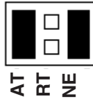
Figure 3-2. Headers J1B – J4B, RS-485 “Auto” Enabled, with “No Echo.”
