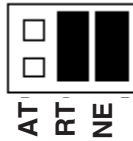
Figure 3-4. Headers J1B – J4B, RS-485 “RTS” Enabled, with “No Echo.”
