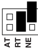
Figure 3-5. Headers J1B – J4B, RS-485 “RTS” Enabled, with “Echo.”
