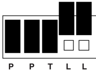
Figure 3-6. Headers J1A – J4A, Line Termination.
