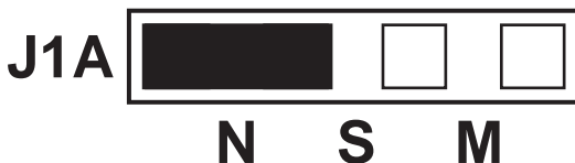
Figure 3-3. Header J1A, normal IRQ mode.
