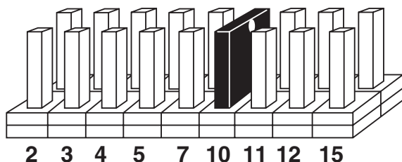
Figure 4-2. Header E1 Optional Windows 3.1 Configuration. IRQ 10 selected. (Refer to Chapter 6 for more information.)
