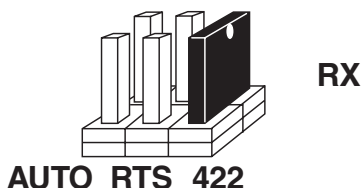
Figure 4-7. This should follow the selection made at E5 if “No Echo” is desired. If Echo suppression is not desired, then leave the jumper in the “422” position. The modem control outputs are only valid when Header E3 is in the 422 mode.
