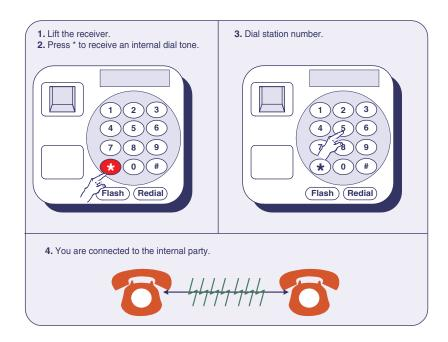
Figure 5-9. Placing an intercom call.
