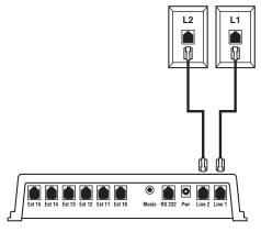
Figure Q-7. Connecting two telephone lines to the Voice Pro, example 2.
