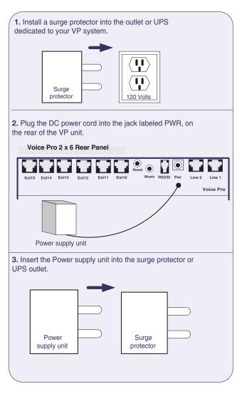
Figure 3-6. Installing a surge protector.
