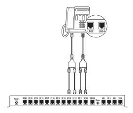
Figure Q-5. Connecting four-line telephones to the Voice Pro.
