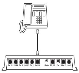
Figure Q-2. Connecting a one-line telephone to the Voice Pro.
