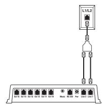
Figure Q-8. Connecting two telephone lines to the Voice Pro, example 3.
