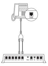
Figure Q-3. Connecting two-line telephones with one jack to the Voice Pro.
