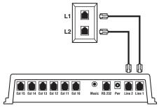
Figure Q-6. Connecting two telephone lines to the Voice Pro, example 1.
