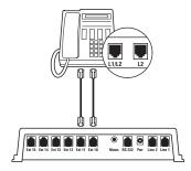
Figure Q-4. Connecting the two-line telephone with two jacks to the Voice Pro.
