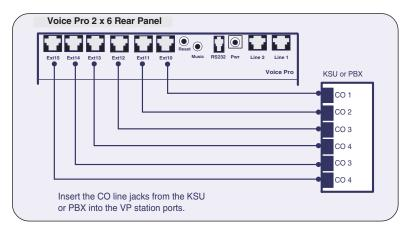
Figure 3-5. Key system or PBX connection.
