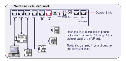
Figure 3-4. Equipment connections.
