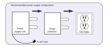
Figure 2-1. Power-supply configuration.
