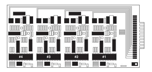
Figure 3-4. The Lineshare Master-4 Circuit Board.
