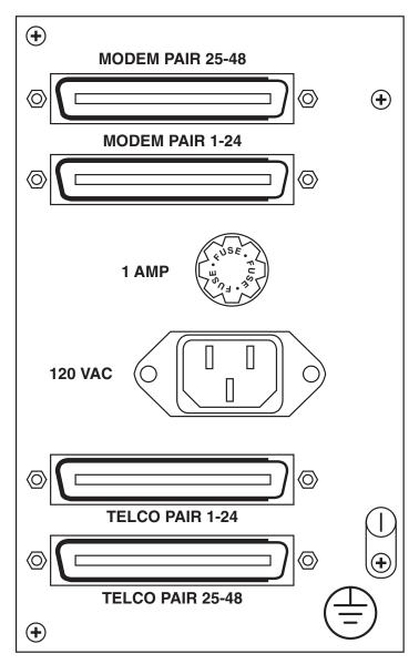
Figure 3-1. Rear Panel of the Lineshare Master-4 Rack.
