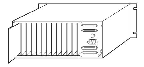
Figure 3-5. The Lineshare Master-4's Removable Circuit Boards.
