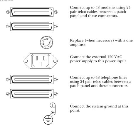
Figure 3-2. Connecting the Telephone Equipment to the Lineshare Master-4.
