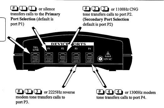
The LineShare Pro 104 will ring the Primary port up to 6 times (Rings to port P1 in this example). If the call remains unanswered after 6 rings, the LineShare Pro 104 will transfer (Automatic No Answer Transfer) the call to the Secondary port. The Automatic No Answer Transfer is designed to accommodate fax machines that do not produce a CNG tone, and can be turned off through programming.
