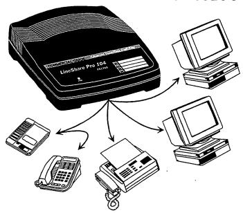
The LineShare Pro 104 is a phone line management system designed to direct incoming phone calls to 1 of 4 destinations. It is capable of transferring calls in virtually any configuration of data devices including, but not limited to the following:
