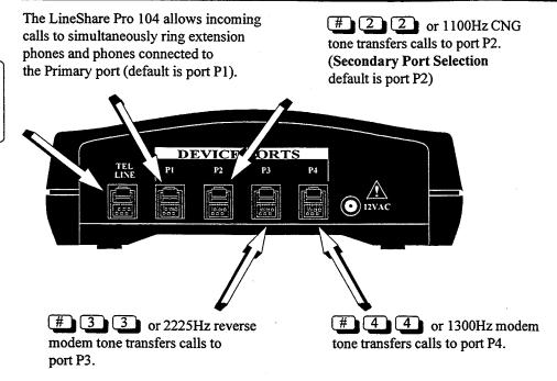
If the LineShare Pro 104 detects any of these signals, it transfers the call to the appropriate port. (The single frequency tones must be detected within the 10 second Single Tone Detection Timer.)
