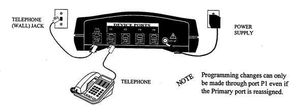
Programming changes can be performed from a tone phone connected to port P1 of an operational unit.
