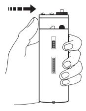
Figure 5-1. Applying thumb pressure to the plastic lens.
