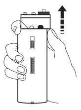
Figure 5-2. Lifting off the plastic lens.
