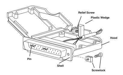
Figure 1. Connector Assembly.
