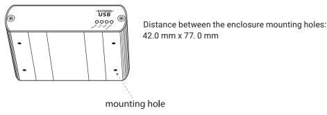
FIGURE 4-2. MOUNTING HOLE ON THE EMD100USB ENCLOSURE
