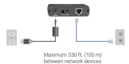
FIGURE QS-3. CONNECT THE REMOTE EXTENDER TO A NETWORK SWITCH
