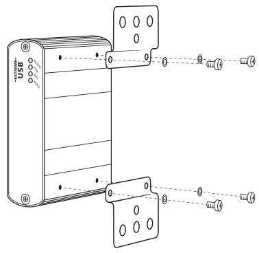
FIGURE 4-1. INSTALLING THE MOUNTING BRACKETS
