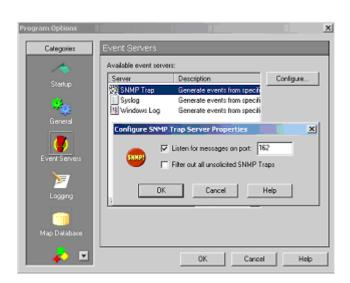
Figure 9 Configure SNMP Trap Server Properties
