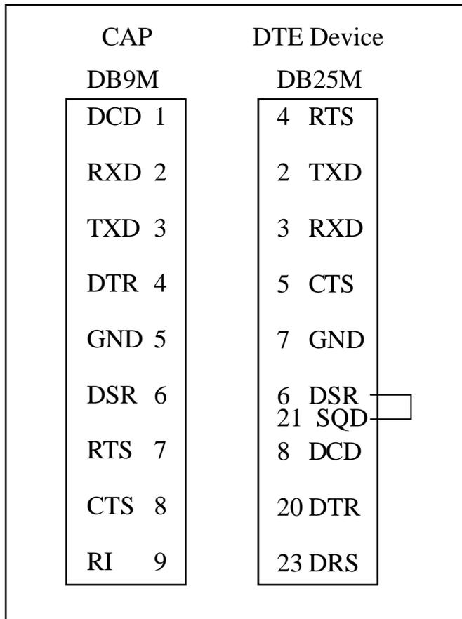
Figure A-1. CAP-to-DTE Cable.
