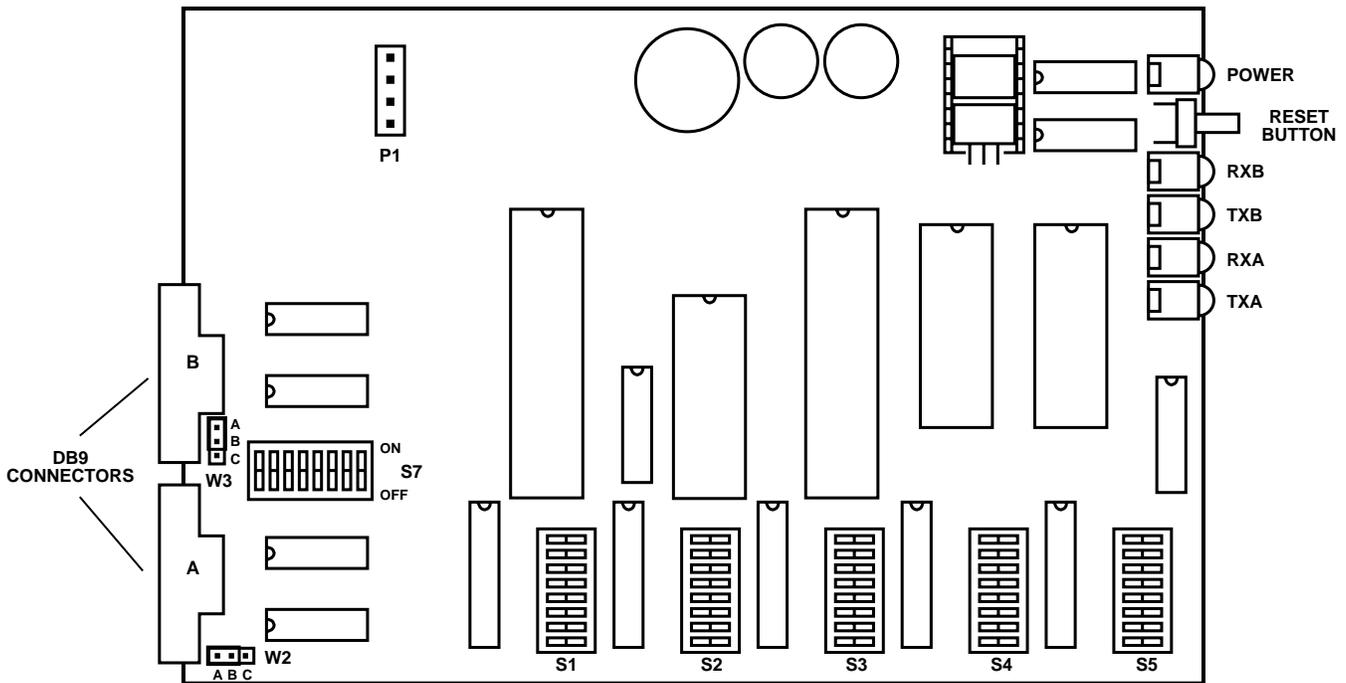
**Figure 3-1. Switch Locations on the Circuit Board.**
