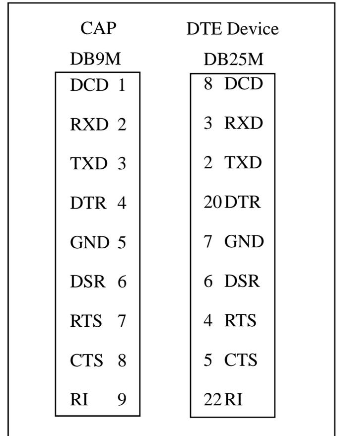
Figure A-2. CAP-to-Modem Cable.
