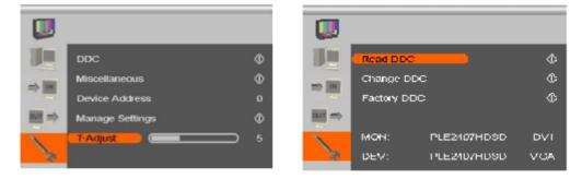
STEP 3: Firstly, READ DDC to copy the EDID info from the transmitter to the VGA to DVI converter and then CHANGE DDC from DVI to VGA to converts the EDID info to VGA
