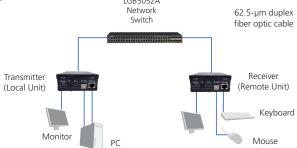
Figure 3-1. Connecting the extender units.
