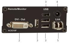
Figure 2-5. ACX310F-R receiver's back panel.
