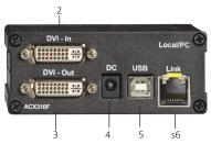
Figure 2-1. ACX310-T transmitter's back panel.
