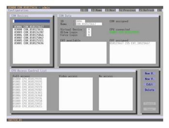
Figure 4-49. Menu Configuration—CON Devices screen.
