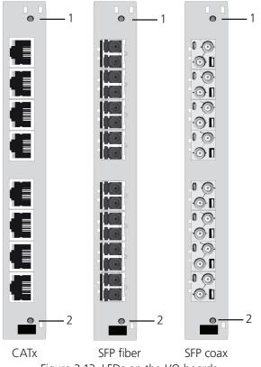
Figure 2-13. LEDs on the I/O boards.
