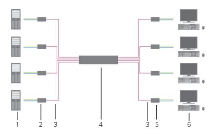
Figure 3-1. KVM using ServSwitch DKM FX application.
