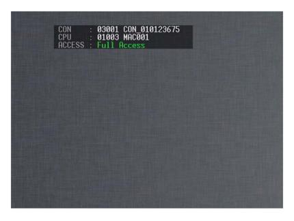
Figure 2-26. Example view of extender OSD.
