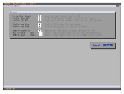
Figure 4-23. Menu Configuration Access screen.
