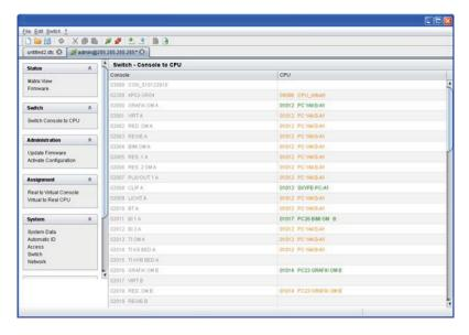
Figure 5-3. Menu Switch—Switch Console to CPU.
