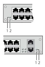
Figure 2-22. Fan Tray Status LEDs on ACXC16, ACXC32, and ACXC48.
