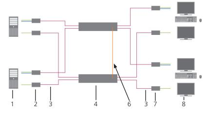
Figure 3-3. Parallel operation (stacking) application.
