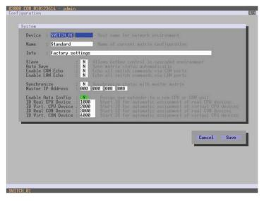
Figure 4-17. Menu Configuration—System screen.
