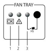
Figure 2-15. Status LEDs on the fan tray.
