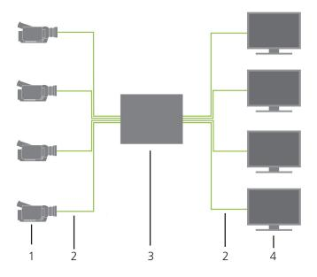
Figure 3-2. Video using ServSwitch DKM FX application.
