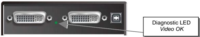
The diagnostic LED 'Video OK' is located near to the CATx/Fibre-connectors
