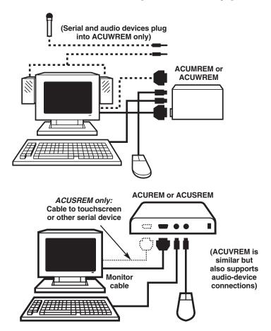
Figure 4-5. Attaching user equipment to a Micro Remote Unit (top) or a fullsize (non-Micro) Remote Unit (bottom, ACUREM or ACUSREM shown).
