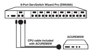
Figure 4-2. Attaching a KVM switch with multiple user-port connectors to a Switching Remote Unit's CPU port.
