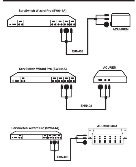
Figure 4-7. Attaching a KVM switch with multiple CPU-port connectors to a Micro Remote Unit (top), a full-size (non-Micro) Remote Unit (middle, ACUREM shown), and an ACU1006MRA Remote Hub (bottom).
