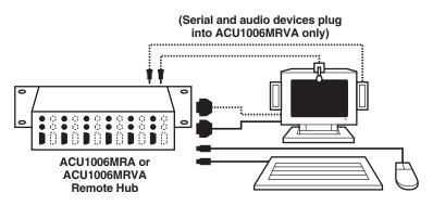
Figure 4-6. Attaching user equipment to a user port on a Remote Hub.
