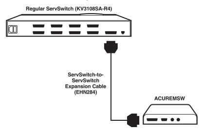
Figure 4-3. Attaching a KVM switch with single ServSwitch style DB25 userport connectors to the CPU port on a Switching Remote Unit's CPU port.
