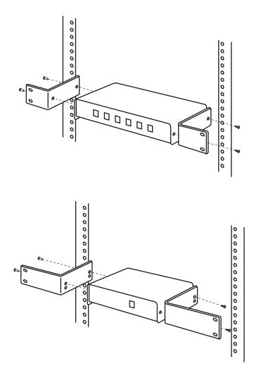
Figure B-2. Mounting the bracketed Remote Hub (above) or Remote Unit (below).
