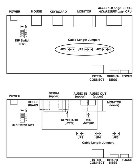
Figure 3-1. The full-size Remote Units' PCBs (main PCB of all but the KVM/Serial/Audio shown at top, main PCB and audio daughtercard of the KVM/Serial/Audio below), showing the jumpers and DIP switch.
