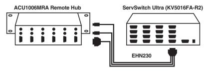
Figure 4-9. Attaching a KVM switch with single composite CPU-port connectors to user-port connectors on a Remote Hub.
