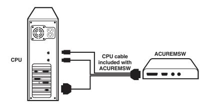
Figure 4-1. Attaching a CPU to a Switching Remote Unit's CPU port.
