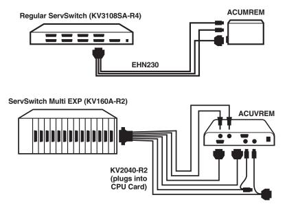
Figure 4-8. Attaching a KVM switch with single composite CPU-port connectors to the user-port connectors on an ACUMREM Remote Unit (top) or any other type of Remote Unit (bottom, ACUVREM shown).
