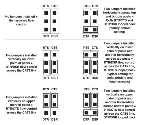
Figure 3-3. Flow-control jumper settings.
