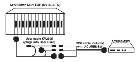
Figure 4-4. Attaching a ServSwitch Multi to the Switching Remote Unit's CPU port.
