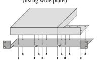
5. Mounting of double width and regular units ( using narrow strip)
