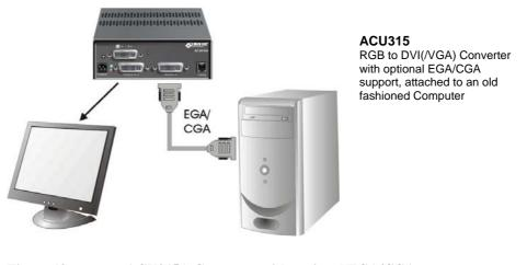
Figure 19 ACU315A Converter with optional EGA/CGA support, attached to an old fashioned Computer
