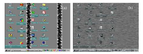
Figure 17 Burst test pattern applied to desktop showing problems with (a) pixel clock setting, (b) pixel phase setting.
