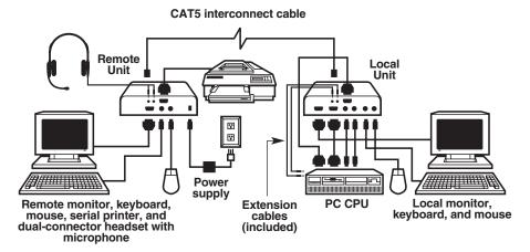
Figure 6-8. A Dual-Access Extender-system installation, rear view.
