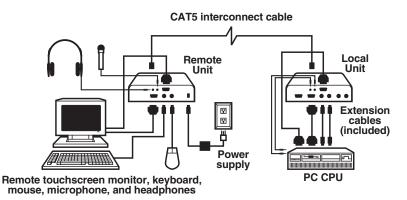
Figure 6-7. A Single-Access Extender-system installation, rear view.
