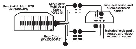
Figure 6-4. Attaching a ServSwitch Multi to the CPU port of a Single-Access Local Unit.
