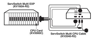
Figure 6-5. Attaching a ServSwitch Multi to the Remote Unit's user port.
