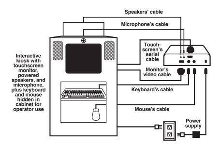
Figure 6-3. Attaching a user station with a monitor, keyboard, mouse, serial device (touchscreen shown), microphone, and speakers to the Remote Unit.
