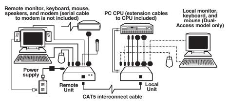
Figure 6-6. An Extender-system installation, front view.
