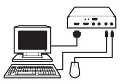
Figure 6-2. Attaching a monitor, keyboard and mouse to the Dual-Access Local Unit.
