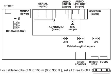
For cable lengths of 100 to 200 m (330 to 655 ft.), set all three to A (
