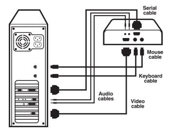
Figure 6-1. Attaching a CPU to the Local Unit (Single-Access model shown).
