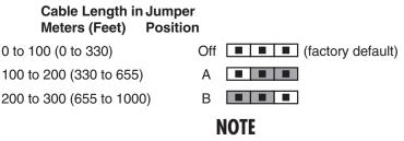
If you will be running cable to near the limit of one of these cable-length ranges, say as far as 80 m (260 ft.), and you will be using high-resolution (1024 x 768 or higher) video, you might be able to achieve more accurate video compensation (see Section 6.4) by selecting the higher cable length range (the 100-to-200-m range in this case).
