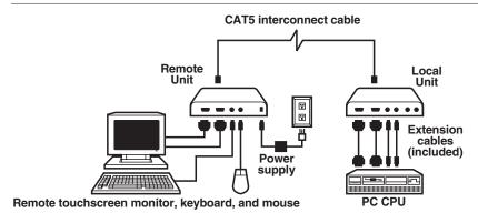
Figure 6-5. A Single-Access Extender-system installation, rear view.
