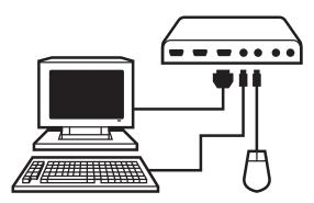
Figure 6-2. Attaching a monitor, keyboard and mouse to the Dual-Access Local Unit.
