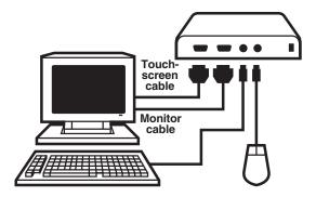
Figure 6-3. Attaching a monitor, keyboard, mouse, and serial device (the monitor's touchscreen shown) to the Remote Unit.
