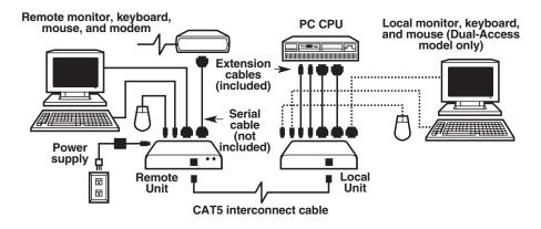
Figure 6-4. An Extender-system installation, front view.
