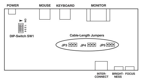
Figure 5-1. The Remote Unit's main PCB, showing the cable-length jumpers and DIP switch.
