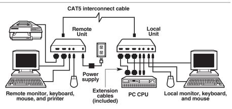
Figure 6-6. A Dual-Access Extender-system installation, rear view.
