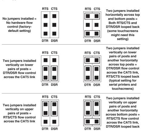
Figure 5-3. Flow-control jumper settings.
