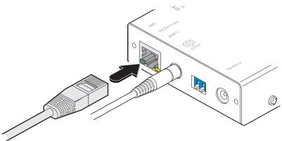
Figure 3-18. Attaching the CATx link cable
