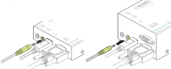
Figure 3-8. Attaching an audio input to the single- and dual-variant local modules
