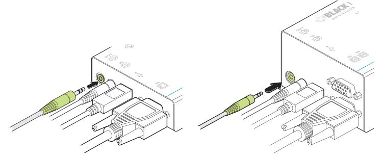
Figure 3-9. Attaching speakers to the single- and dual-variant local modules
