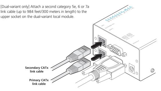
Figure 3-11. Attaching two CATx link cables to a dual-variant local module
