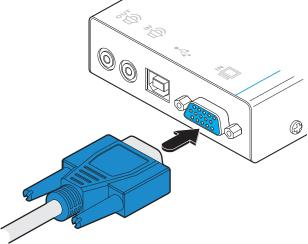
Figure 3-3. Attaching the VGA video link cable
