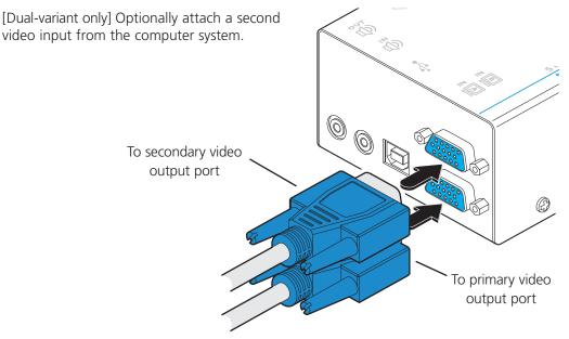
Figure 3-4. Attaching two VGA video link cables to the dual-variant local module
