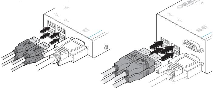
Figure 3-16. Attaching the keyboard, mouse and other USB cables
