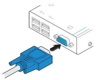
Figure 3-14. Attaching the VGA video display cable
