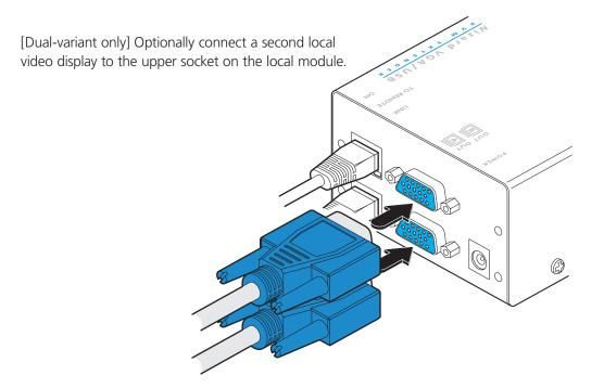
Figure 3-6. Attaching two VGA video displays to the dual-variant local module
