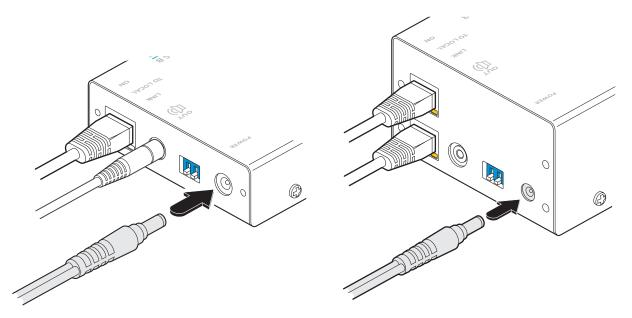
Figure 3-20. Attaching the power adapter
