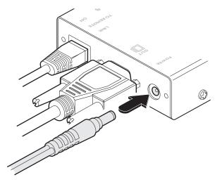
Figure 3-12. The use of a power supply on single-variant local modules is optional. Dual-variant local modules always require a power supply.
