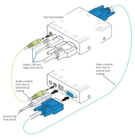
Figure 3-23. Interconnections required for a dual user configuration
