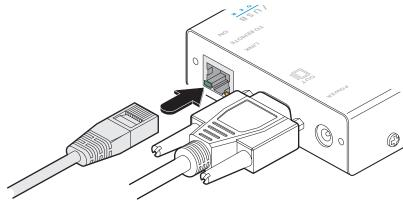
Figure 3-10. Attaching the CATx link cable
