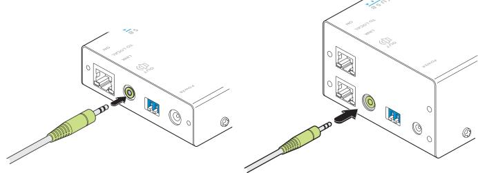
Figure 3-17. Optionally attaching stereo speakers
