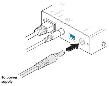
Figure 3-11. Attaching the power adapter
