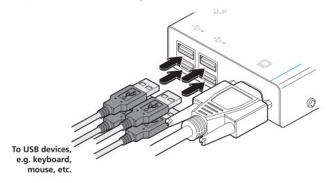
Figure 3-8. Attaching the keyboard and mouse USB cables
