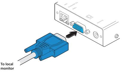
Figure 3-5. Optionally attaching a local video monitor
