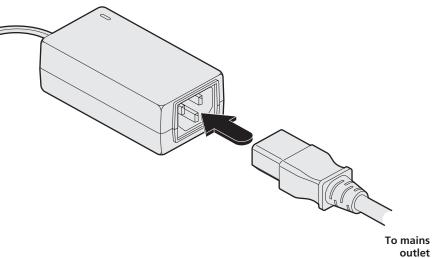
Figure 3-12. Attaching the power cord to the adapter
