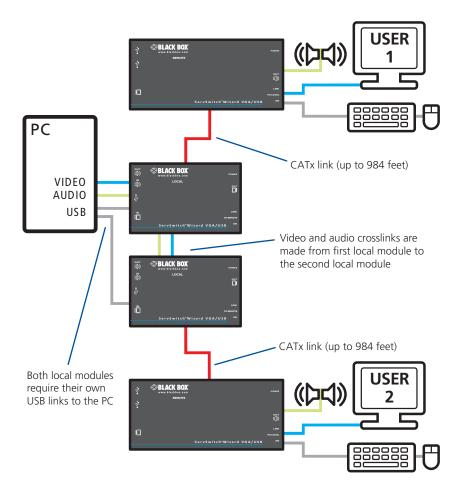
Figure 3-13. The logical layout of a dual user configuration
