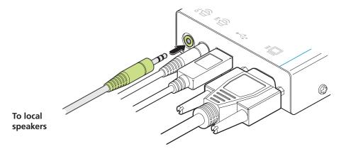
Figure 3-4. Optionally attaching local speakers
