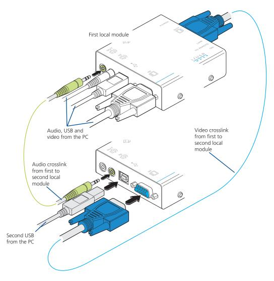
Figure 3-14. Interconnections required for a dual user configuration
