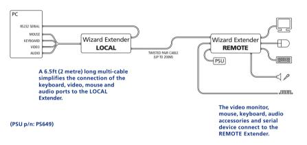
Internal circuitry within the remote module ensures crisp video images by automatically compensating for the length of the twisted pair cable run.
