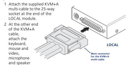
connectors to the appropriate sockets at the rear of the computer system. On most systems the appropriate ports should be labelled and color coded in a similar way to the cable connectors:
