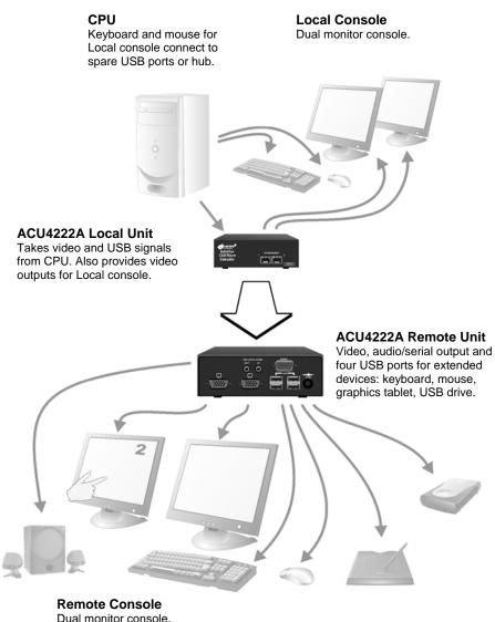
Dual monitor console. Monitor 2 is serial touch screen.
