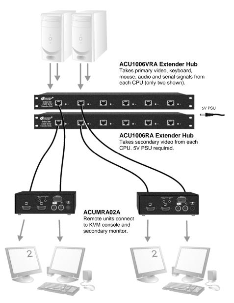
Figure 7 Dual-monitor consoles with serial and audio extension
