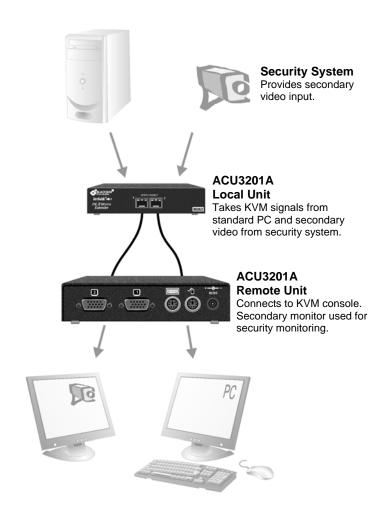
Figure 9 Extender system using ACU3201A kit with second screen for security monitoring
