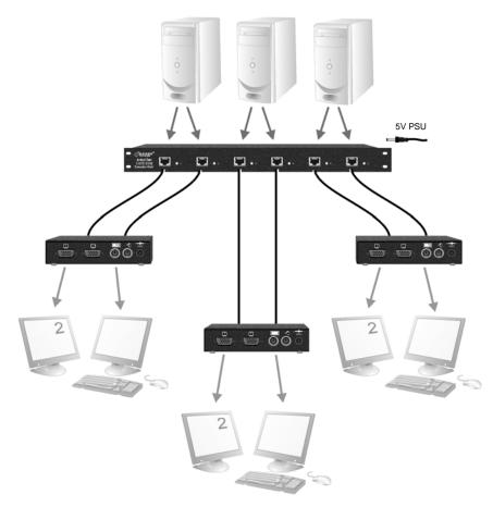
Figure 6 ACU1006RA rack used with ACUMR02A Remote Units to extend dual video
