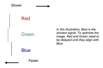
Figure 8 Illustration of skew and appearance on test card
