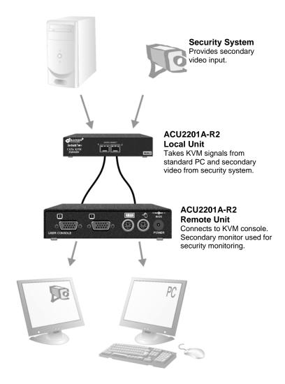
Figure 10 Extender system using ACU2201A-R2 kit with second screen for security monitoring
