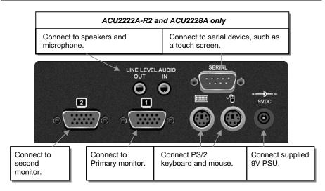
Figure 2 Remote Unit – rear view
