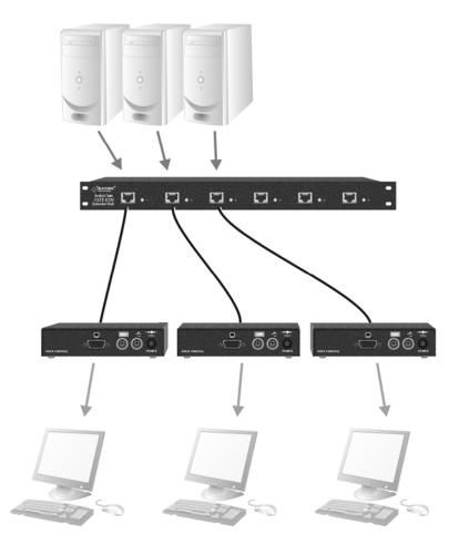
Figure 10 Simple system using ACU1006RA hub and ACUR001A Remote Units
