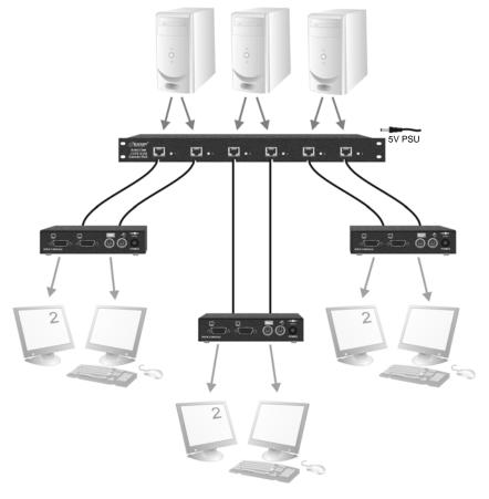
Figure 11 ACU1006RA rack used with ACUR002A Units to extend dual video
