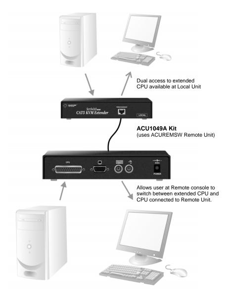
Figure 13 ACU1049A kit with switching Remote Unit
