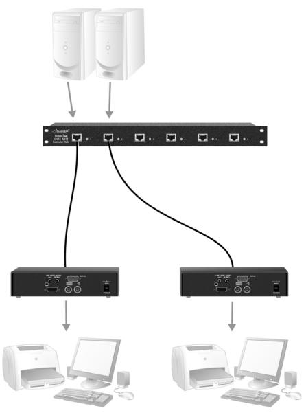
Figure 8 Simple system using ACU1006VRA Hub and ACUVREM Remote Units to extend audio, serial and KVM for up to six PCs
