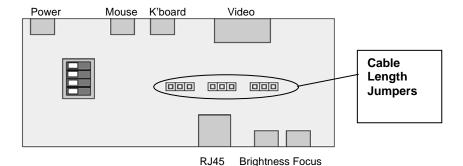
Figure 2 Location of cable length jumpers on Remote Unit's main circuit board
