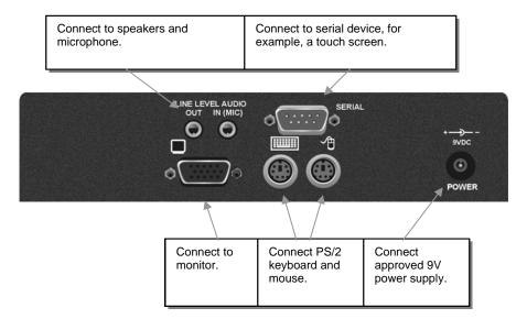
Figure 4 Audio Remote Units (ACUVREM – also supplied with ACU1022A and ACU1028A kits) – rear view
