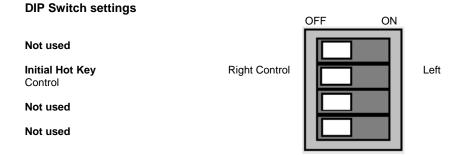
Figure 10 Remote Unit DIP switches on Audio/Serial/Switching CAT5/5e KVM Extenders
