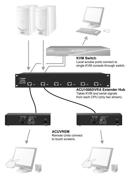
Figure 11 Touch screen network with local access to CPUs through KVM switch.
