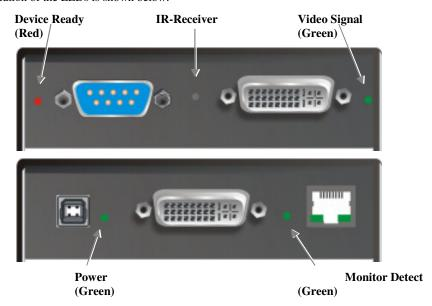
Figure 1 Diagnostic LEDs on RGB to DVI(/VGA) Converter
