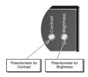
On each ACS335A KVM-Extender you can adjust Brightness and Contrast manually. You'll find the potentiometers to the right hand of the fibre connectors at the remote unit. Please use these potentiometers for a common adjustment of all colours simultaneously. Use these possibilities for normal adjustments.
