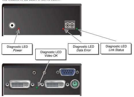
Diagnostic - LEDs at DVI-D KVM Extender
