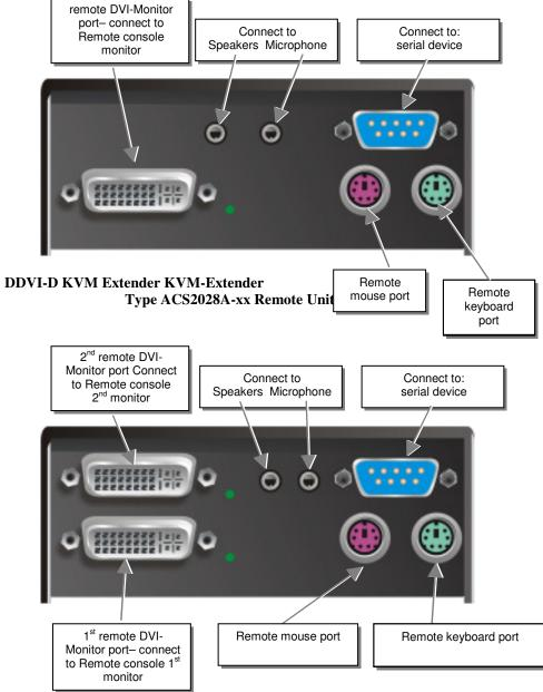
DVI-D KVM Extender KVM-Extender Type ACS2228A-xx Remote Unit
