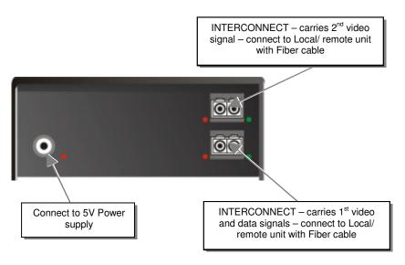
DVI-D KVM Extender KVM-Extender Type ACS2228A-xx Local/ Remote Unit
