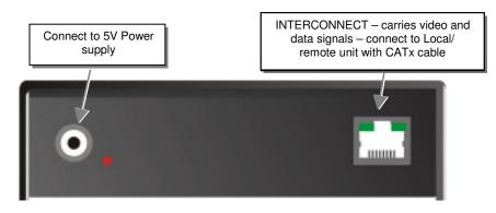
DVI-D KVM Extender KVM-Extender Type ACS1009A Local/ Remote Unit
