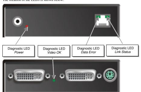
Diagnostic - LEDs at DVI-D KVM Extender
