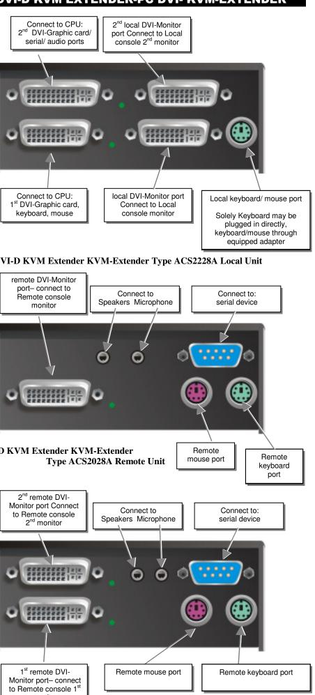
DVI-D KVM Extender KVM-Extender Type ACS2228A Remote Unit
